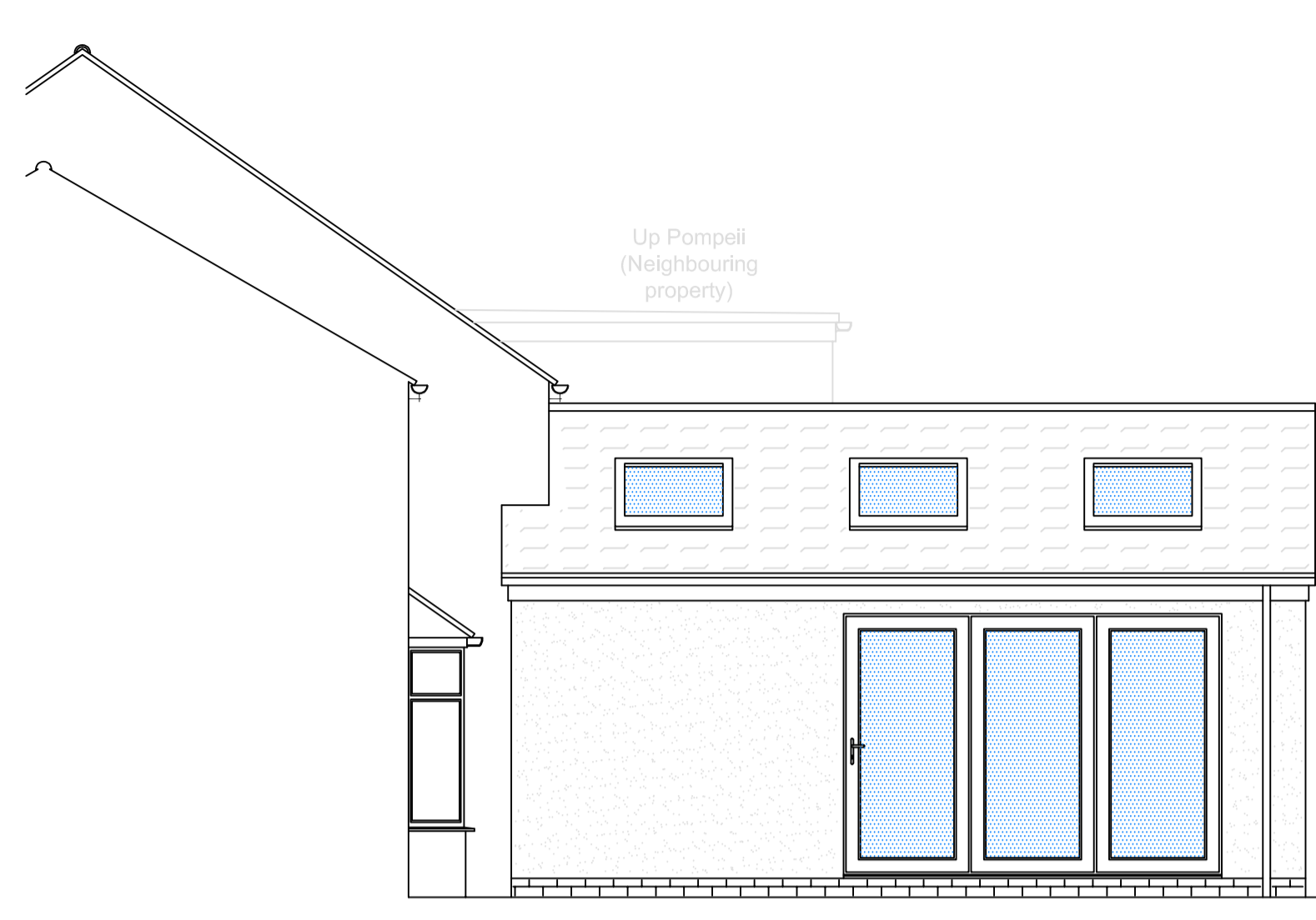
SIDE EAST ELEVATION PROPOSED - SCALE 1:50
