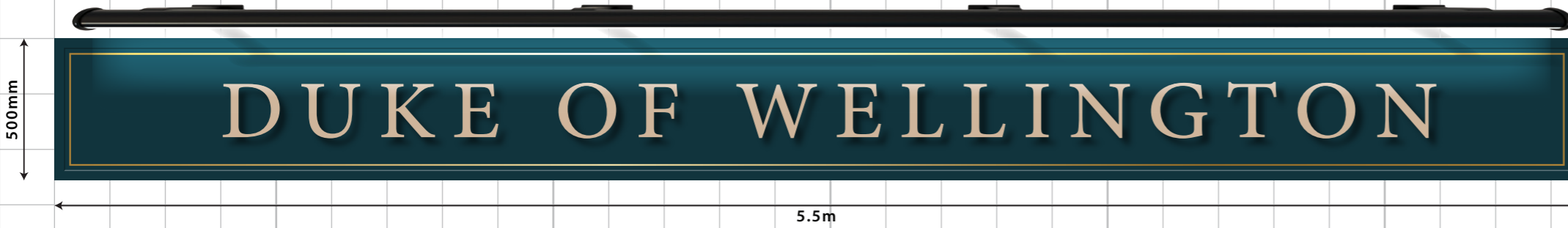
A ONE X NEW FASCIA WITH APPLIED LETTERS AND NEW TROUGH LIGHT SIZE. 5.5m x 500mm. H.A.G. 2.6m.
