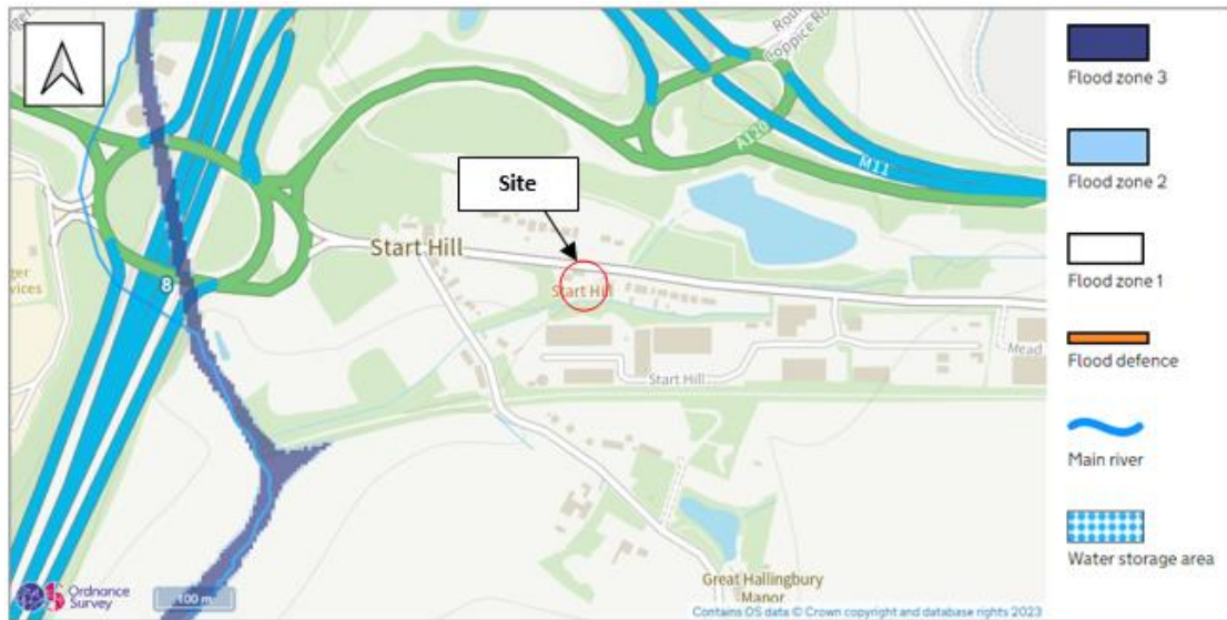
Figure 4-1: Indicative Fluvial/Tidal Floodplain Extent
