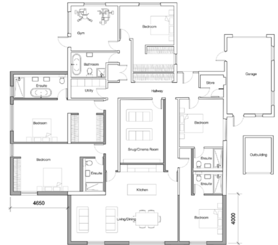
Proposed ground floor plan. Dark grey hatch illustrates extended walls.
