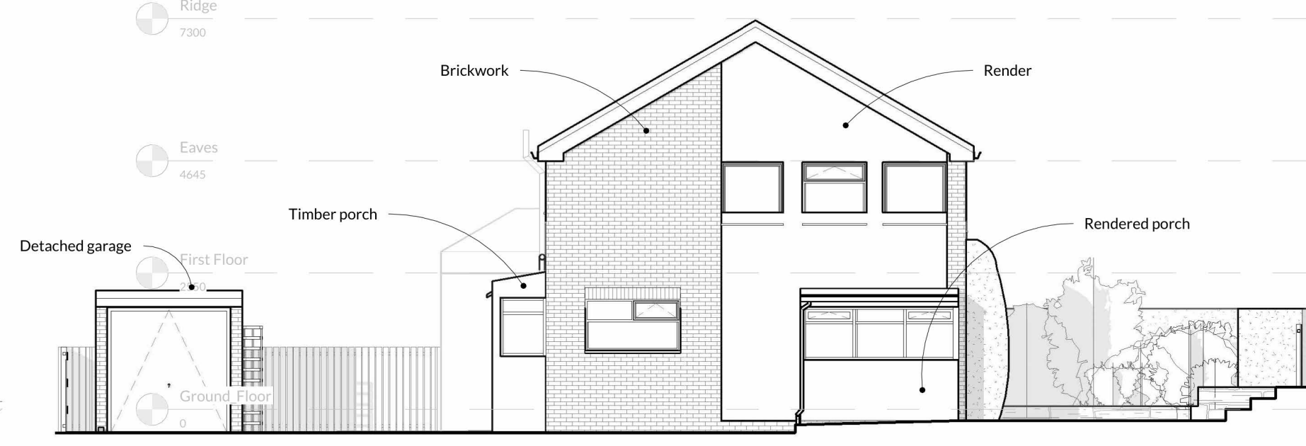
02 - West Elevation (Side) 1: 100
