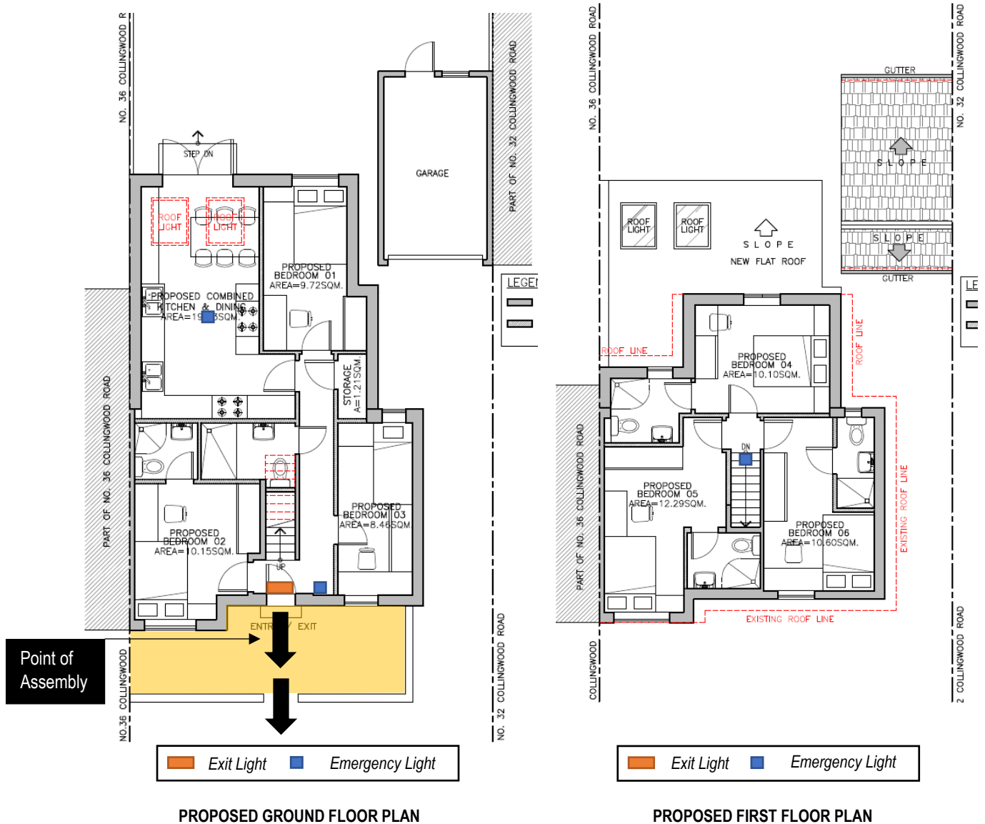
Proposed Floor Plans showing the location of emergency, exit lights and evacuation strategy
