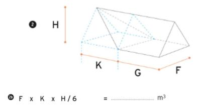
The calculation would therefore be:  $5.284 \times 1.974 \times 2.274/6 = 3.953m3$  (plus 1.45m3)
