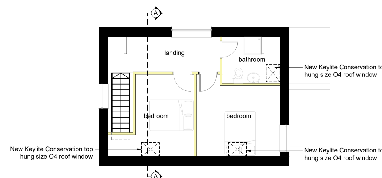
Proposed First Floor Plan (1:100)
