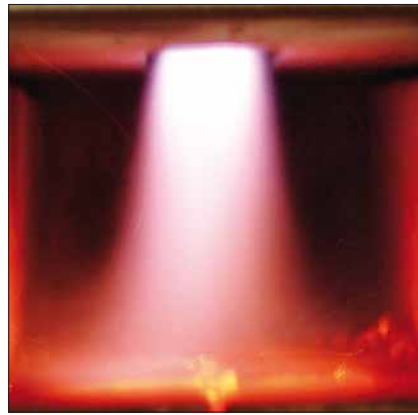
complete combustion of the wood gases in the lower combustion chamber
