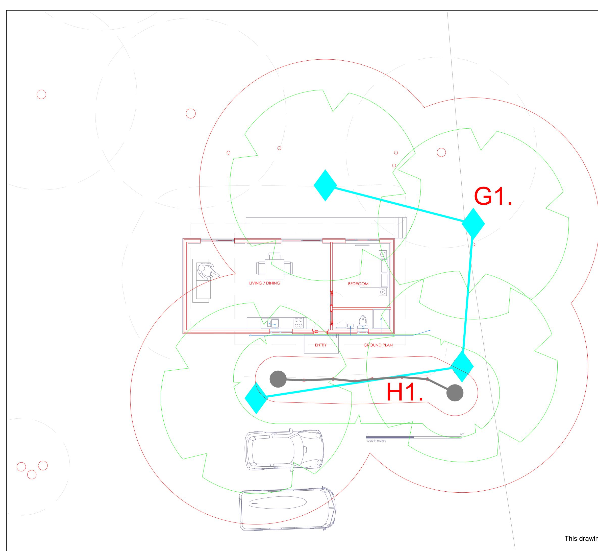
1, Tree Root Protection Areas have been added to survey drawing as supplied.
