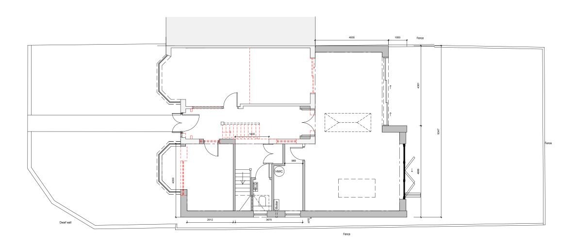
Proposed Ground floor plan showing demolitions 1:100
