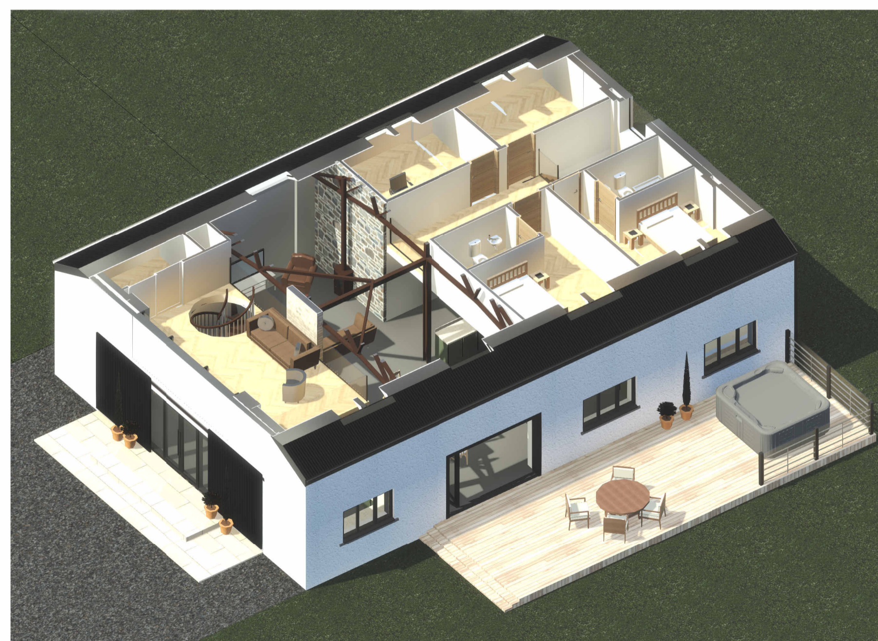
First Floor/ Mezzanine 3D Section
