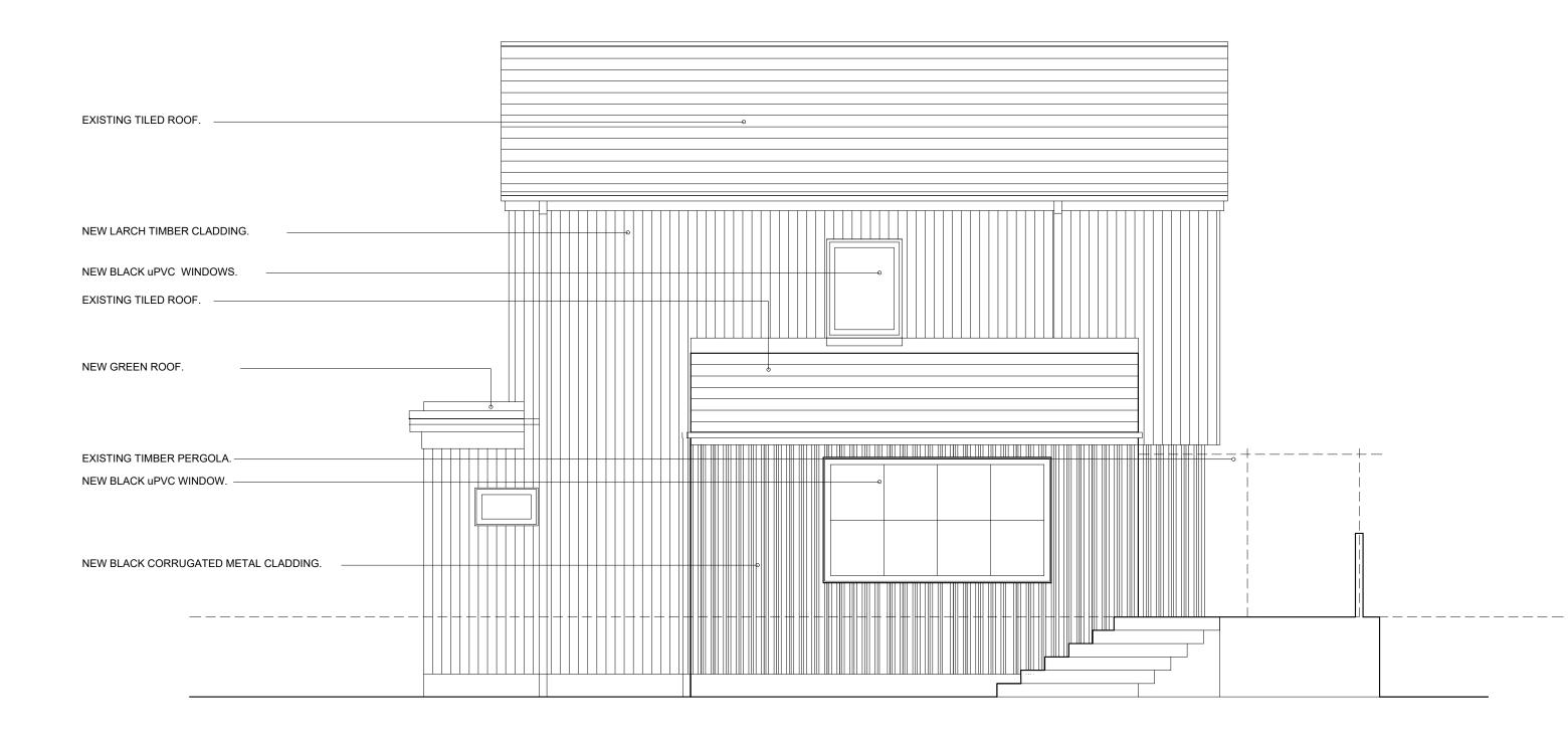
PROPOSED side (SOUTH) elevation 1/50 @A3
