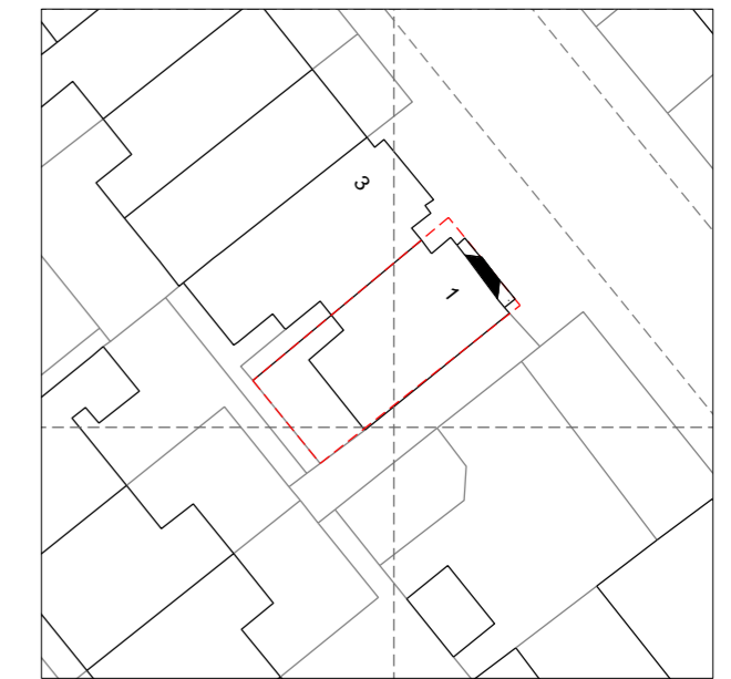
Block Plan 1:500 - new works shown red and dashed
