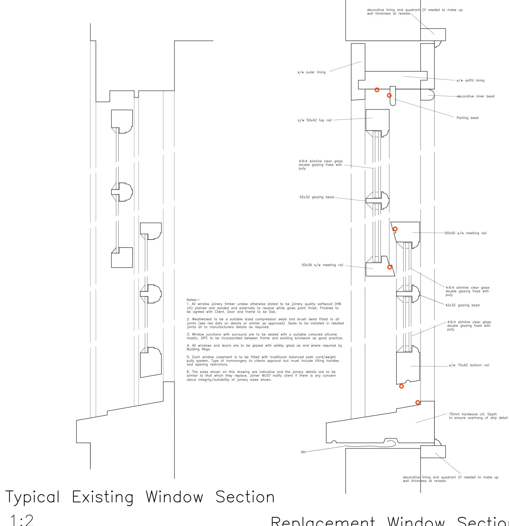
1:2 Scale Bar O Locations of brush or compressible draft seals 200 500 mm 300  $\bigcirc \bigcirc \bigcirc$ 400
