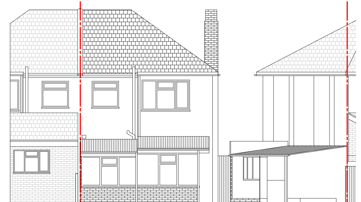
EXISTING REAR ELEVATION
