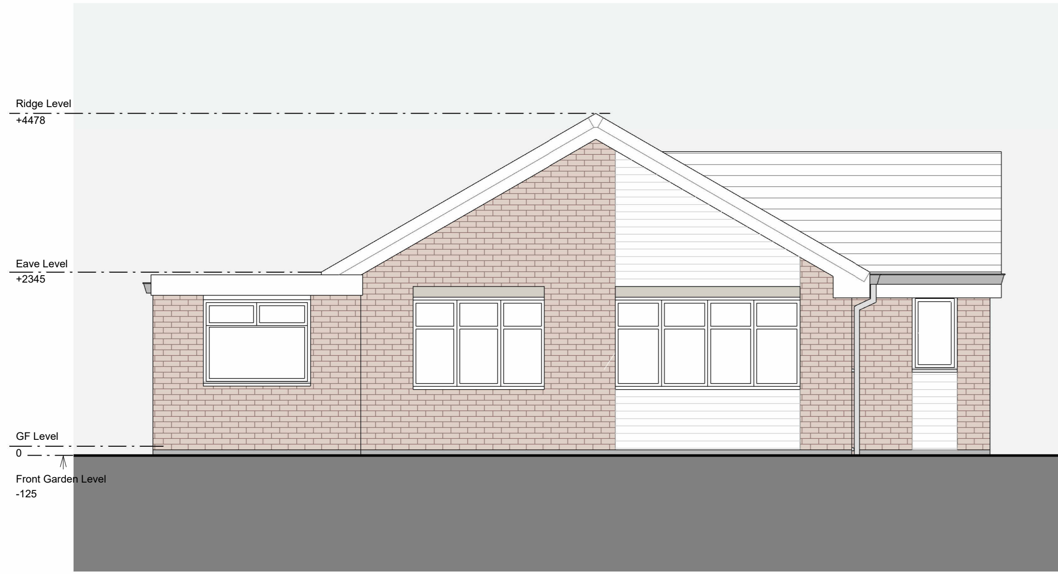
1 EXISTING FRONT ELEVATION 1 : 50
