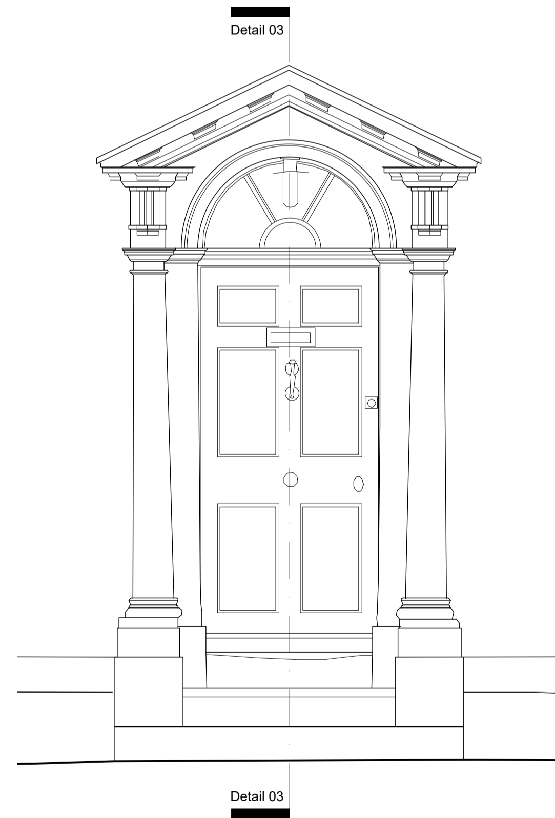
Detail 02 (Elevation) Scale 1:20
