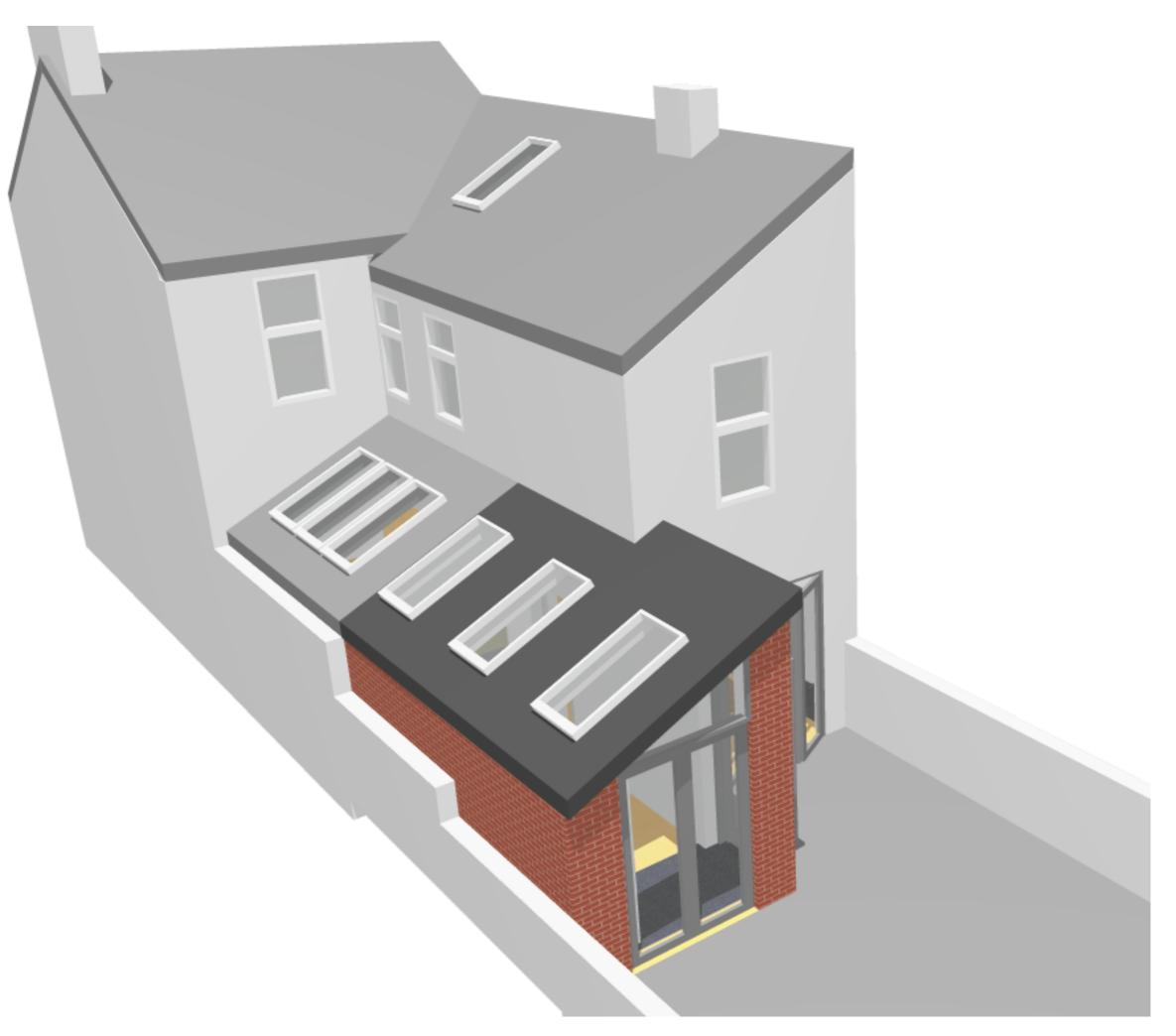
'B' - Velux rooflight added to First Floor
