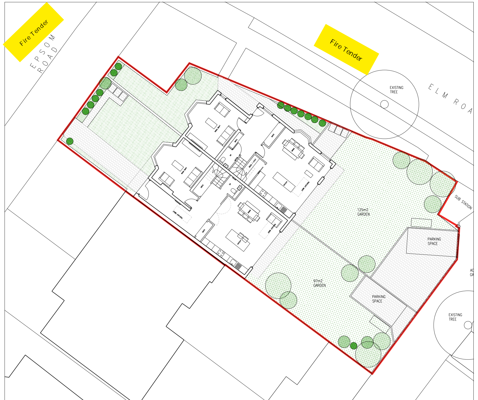
Site Plan showing fire tender position along either Epsom Road and Elm Park West
