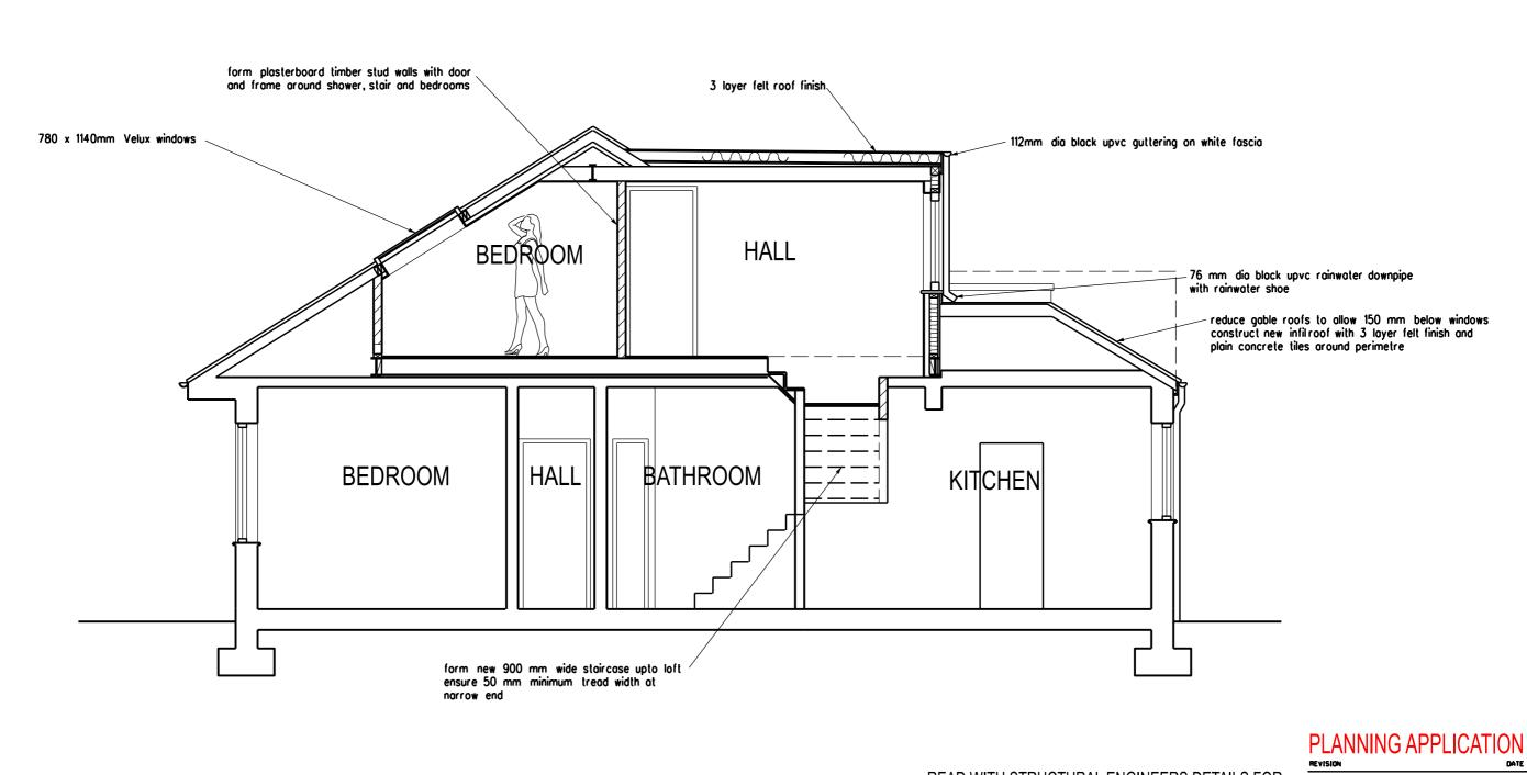
READ WITH STRUCTURAL ENGINEERS DETAILS FOR BEAMS, DORMER, JOISTS & PADSTONES
