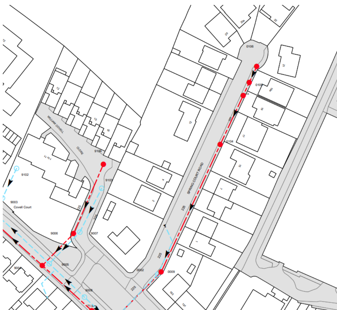
Figure 4.1: TWU Sewer Record Extract
