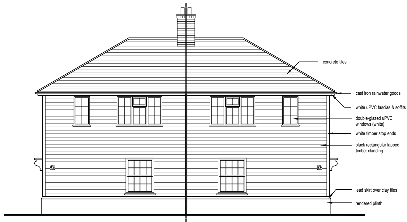
Existing Front Elevation (North East)
