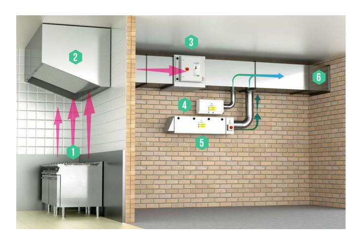
For optimum performance we would recommend between 2 & 6 seconds of dwell time to allow the ozone to work effectively upon the malodorous gasses within the duct.
