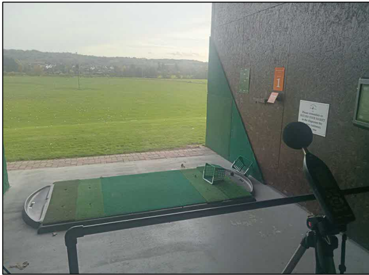
FIGURE 4.2: PHOTOGRAPH OF SOURCE-TERM ATTENDED MONITORING EQUIPMENT
