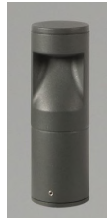
Figure 4: Example of downwards shielded bollard light. This particular example is the LAKO 7W 3000k LED ground bollard, IP65, 173 lumens, or equivalent style of fitting
