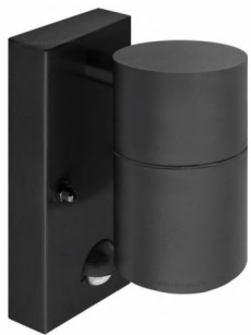
Figure 6: Example of proposed downwards shielded wall light with PIR sensor. This example is 'Black PIR stainless steel single outdoor wall light with movement sensor down ZLC037DSEN' The lamp is not included, so a 2100—3000K 5W LED lamp can be installed. The sensor can be adjusted up to max 8m x 8m, the timer adjusted from 5 sec—5 mins to give a good level of control.
