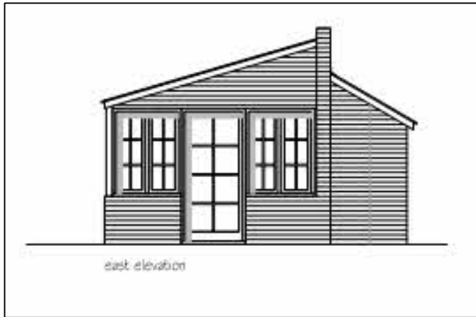
East elevation of proposed garden office.
