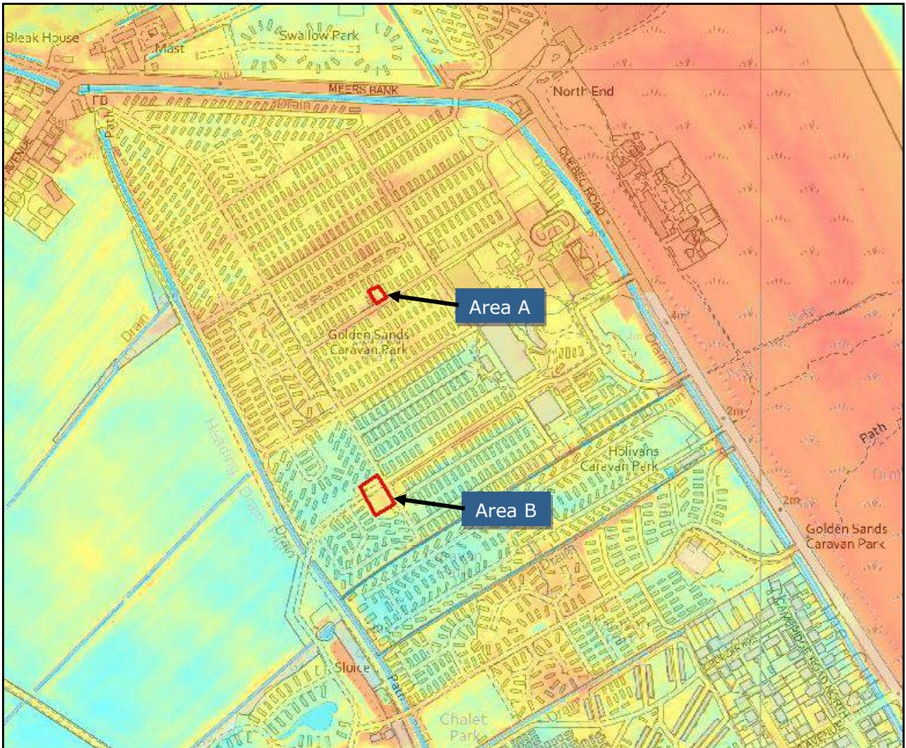
Figure 2: Filtered LIDAR survey data at 1m resolution where higher ground is denoted by red and orange colours and lower ground is denoted by blue colours
