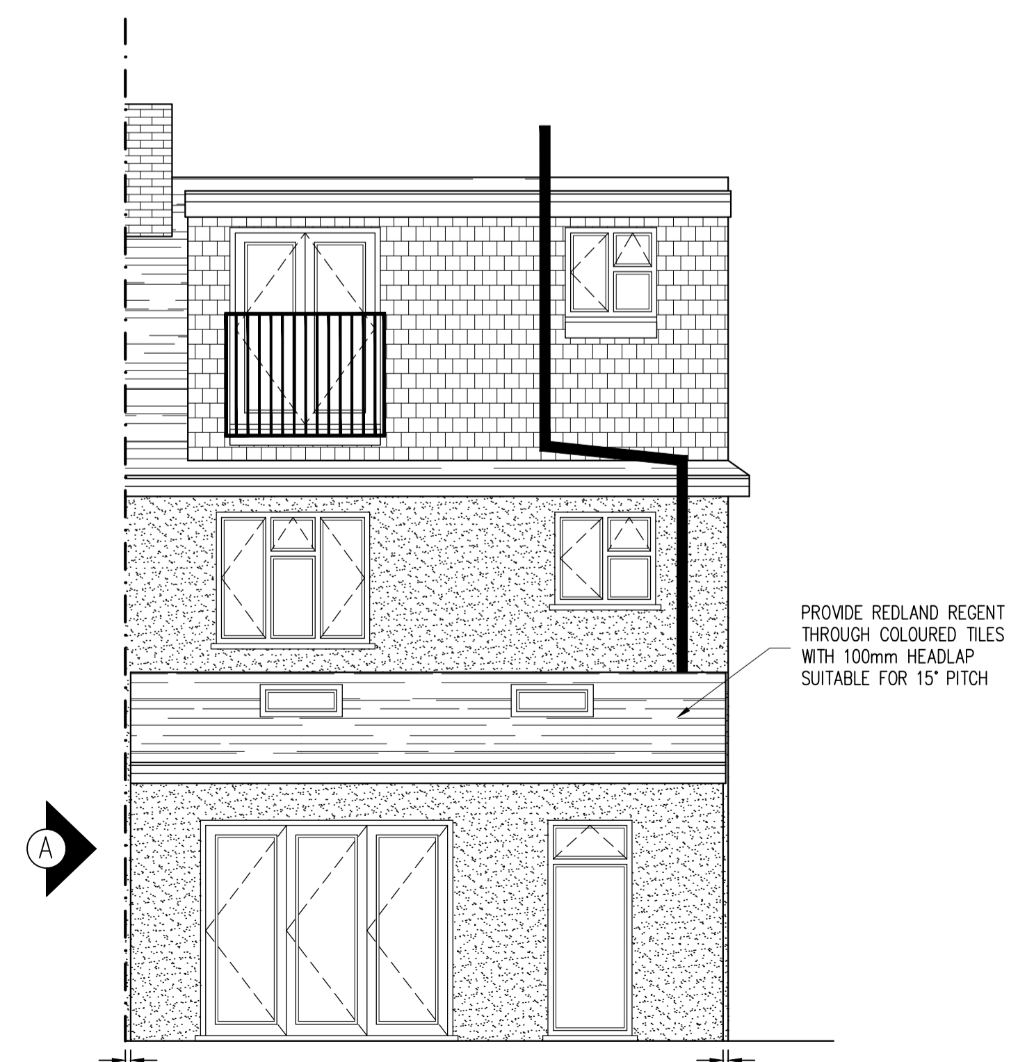
PROPOSED REAR ELEVATION SCALE 1:50
