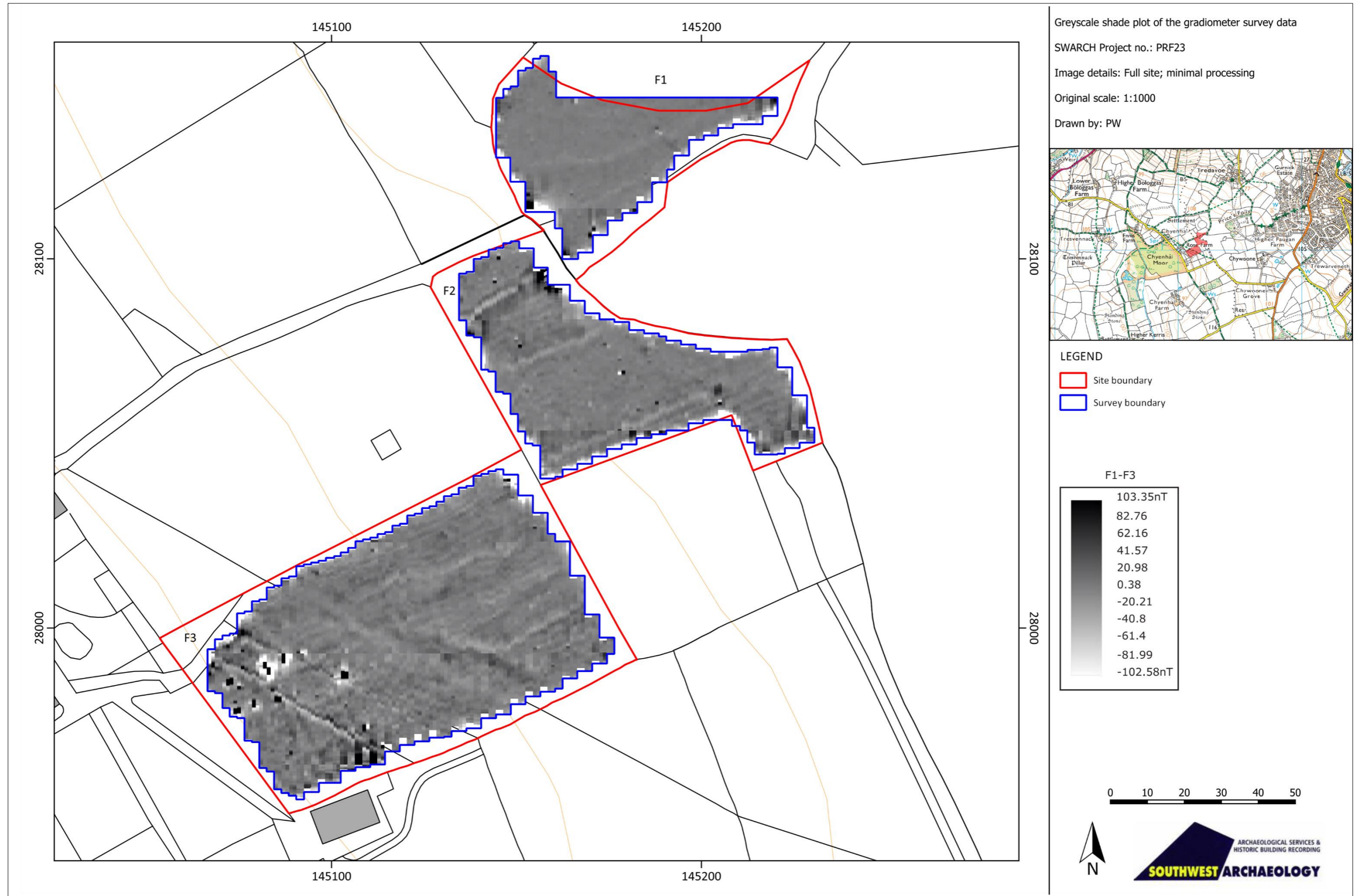
FIGURE 3: GREYSCALE SHADE PLOT OF THE GRADIOMETER SURVEY DATA; MINIMAL PROCESSING (CONTAINS ORDNANCE SURVEY DATA © CROWN COPYRIGHT 2023. LICENCE NUMBER 100022432).
