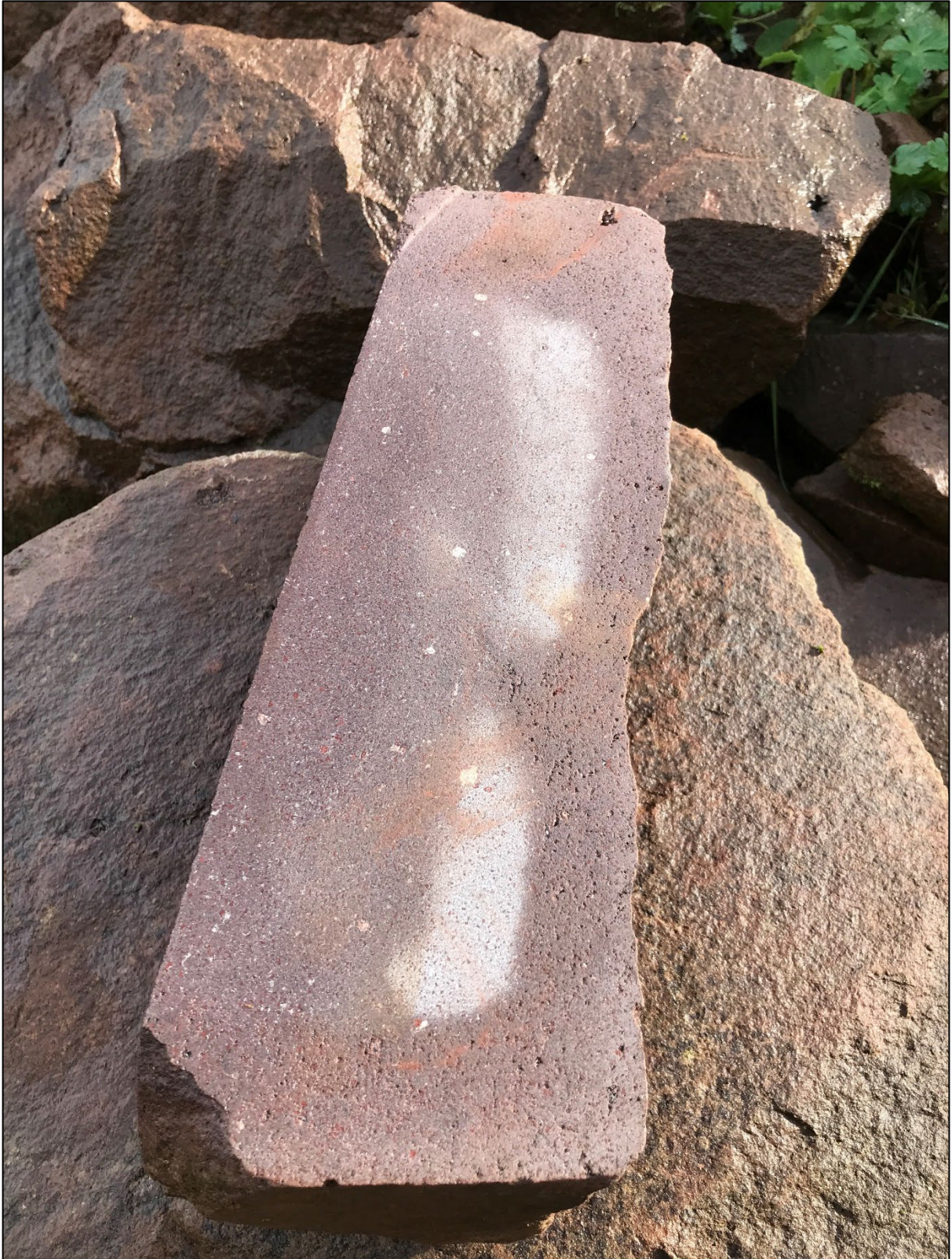
Photo 3: The new floor within Room 1 will utilise volcanic flagstones sourced from a local quarry. These would be consistent with existing in-situ historic flagstones (Fig. 1, 1)
