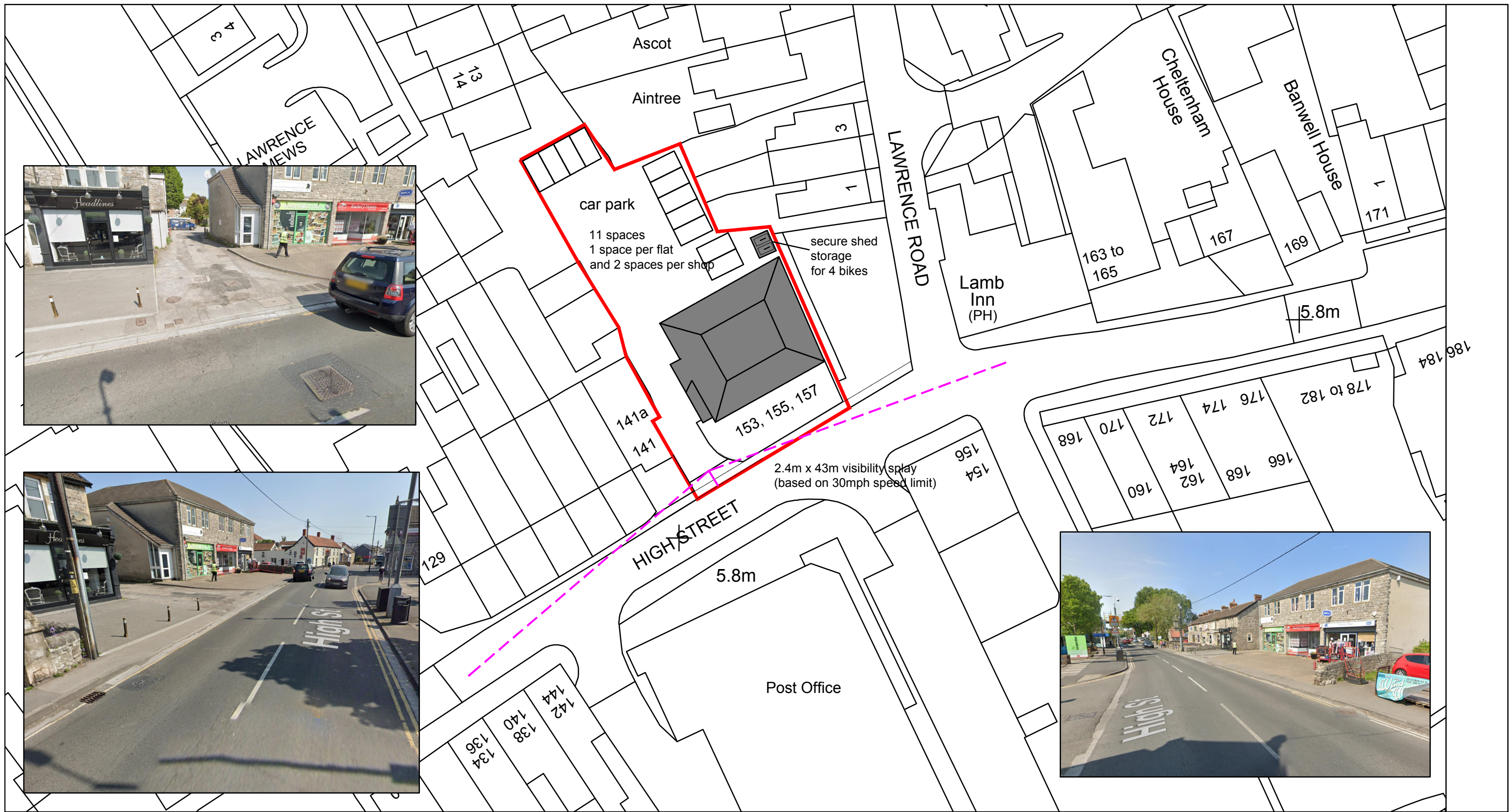
SITE PLAN WITH 2.4M X 43M VISIBILITY SPLAYS
