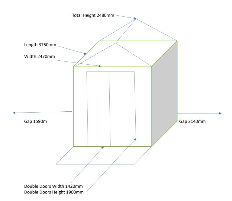
Existing materials: External – wood – painted in pale green Roof - wood with felt overlay Decked areas– paving slabs
