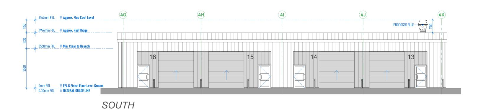
PROPOSED FLUE 45 43 PROPOSED FLUE 6147mm FGL ▼ Approx. Flue Cowl Level 6147mm FGL Approx. Flue Cowl Level 4996mm FGL **V Approx. Roof Ridge** 4996mm FGL **V Approx. Roof Ridge** 3560mm FGL ▼ Min. Clear to Haunch 3560mm FGL ▼ Min. Clear to Haunch 13 -16 9 -12 Omm FGL FFL.G Finish Floor Level Ground
