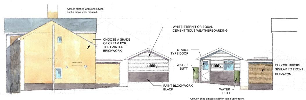
Collect rainwater off roof into two water butts before
