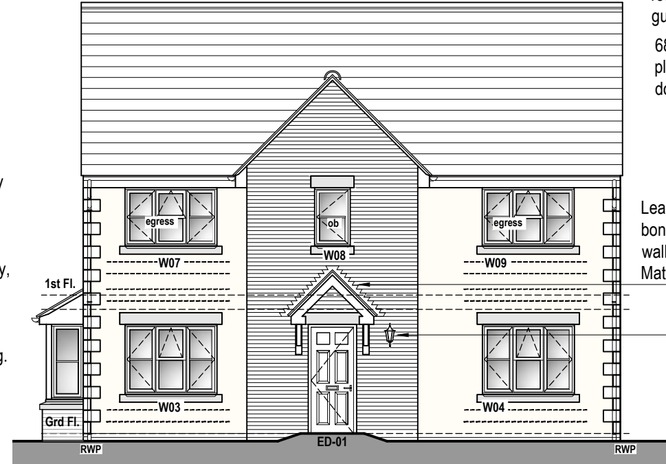
Disabled 'LEVEL' access to door D-01, refer separate details FRONT ELEVATION (Street Elevation)
