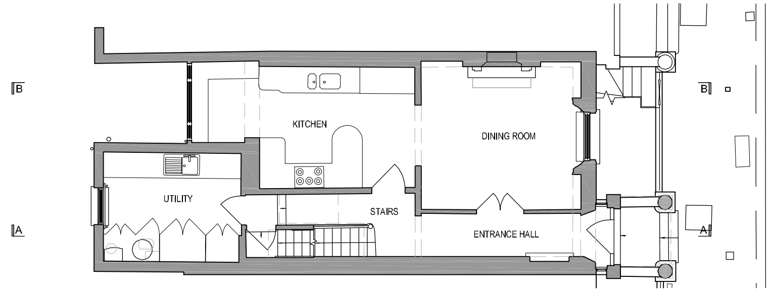
2 GROUND FLOOR PLAN - AS EXISTING Scale: 1:100
