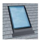
Slim line frame for pitched roof. Reset within roof tilies. Can be fixed to roof pitch as low as 12 deg. & as high as 90 deg.
