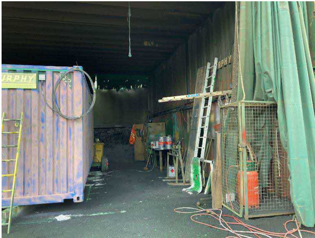
Photograph 7: The old shotblasting unit, located in the central south of the depot area. The floor is regularly scraped and paint flecks are put into skips.
