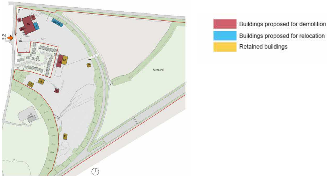
Figure 3-1 - Existing site demolition plan
