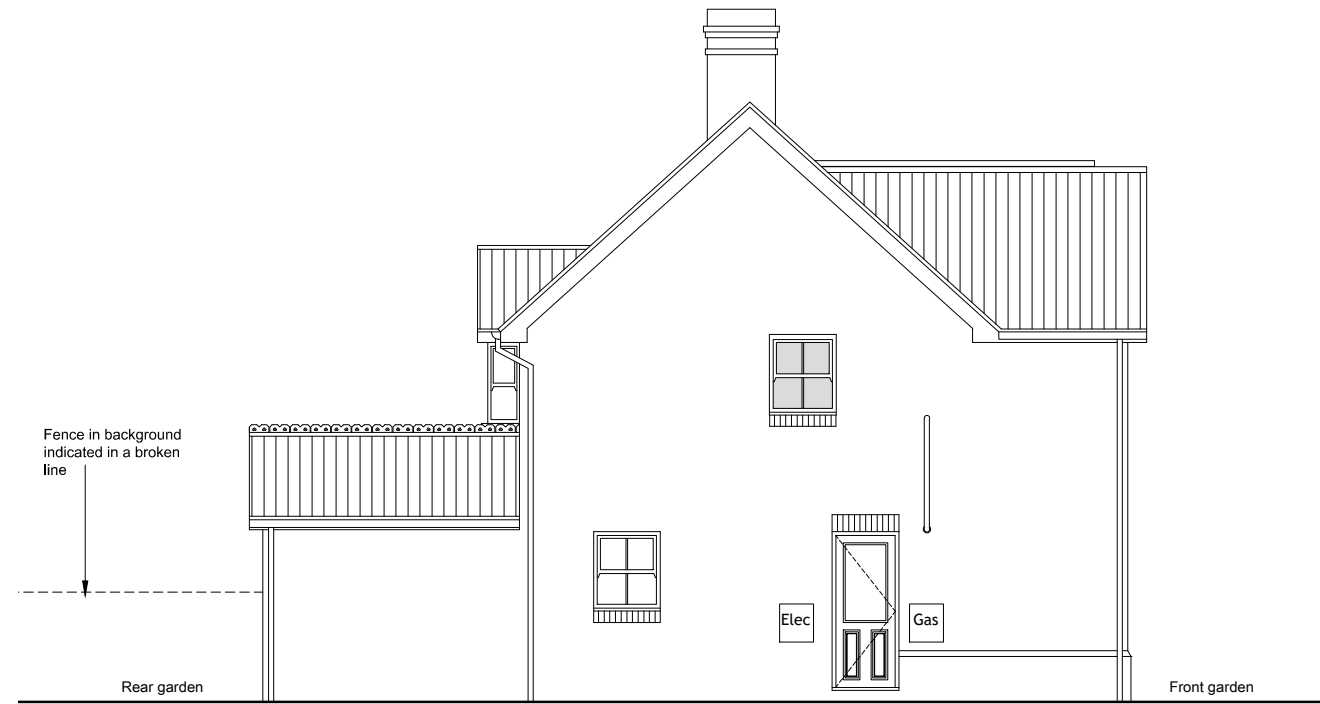
EXISTING SIDE ( E ) ELEVATION 1:100
