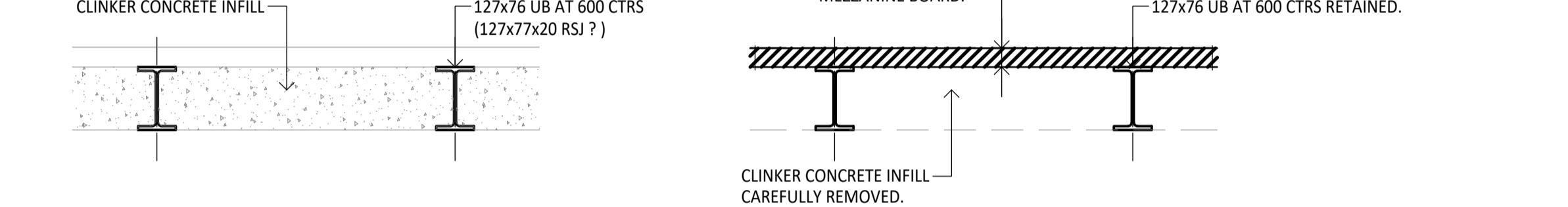
TYPICAL SECTION THROUGH CLINKER/STEEL JOIST FLOOR. / TYPICAL PROPOSED SECTION THROUGH CLINKER/STEEL JOIST FLOOR.
