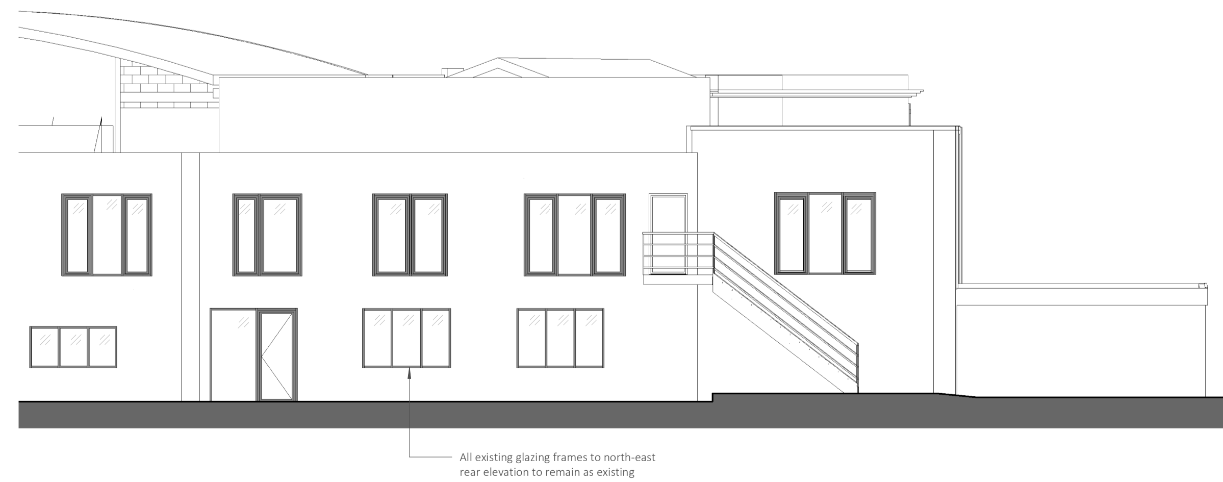
6 - Proposed Showroom Rear Elevation (north-east) 1 : 100
