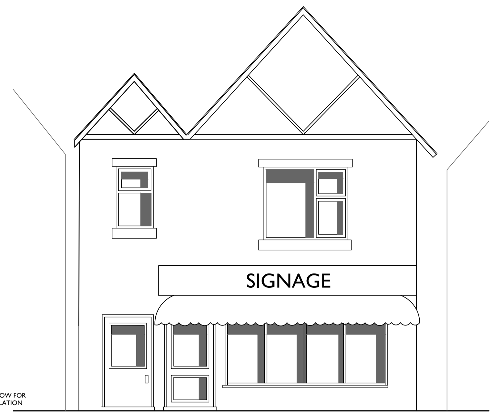
SHOP FRONT ELEVATION AS PROPOSED (FOR PLANNING USE ONLY—DO NOT USE FOR CONSTRUCTION) (SCALE 1:50@A1)
