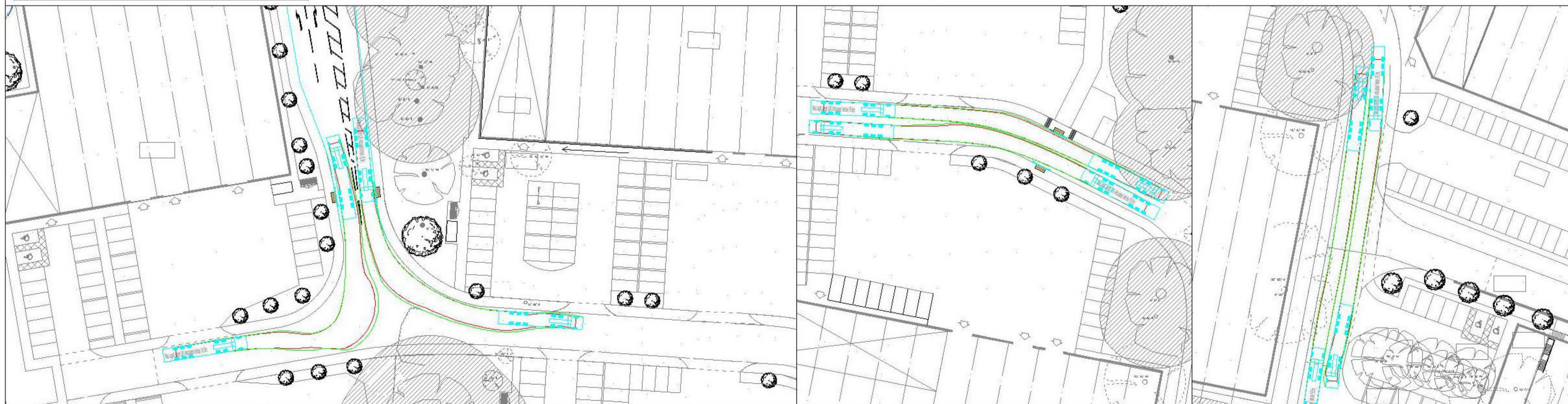
ACCESS ROAD TRACKING (SCALE 1:1000)
