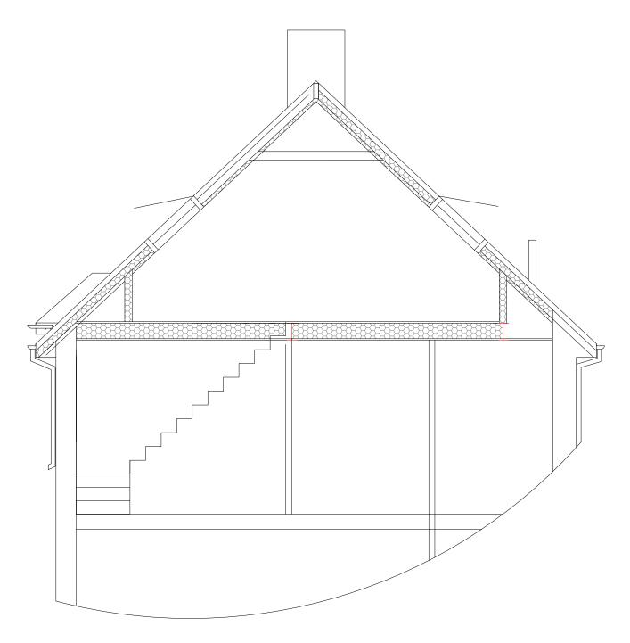
**Cross Section of The Stairs into the** Conversion
