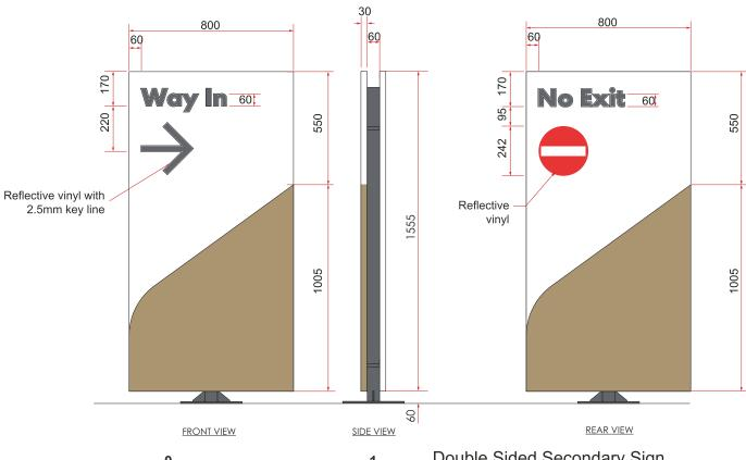
Double Sided Secondary Sign Aluminium from panels painted white and Shell Teal, fitted to MS post with sign fix channel.
