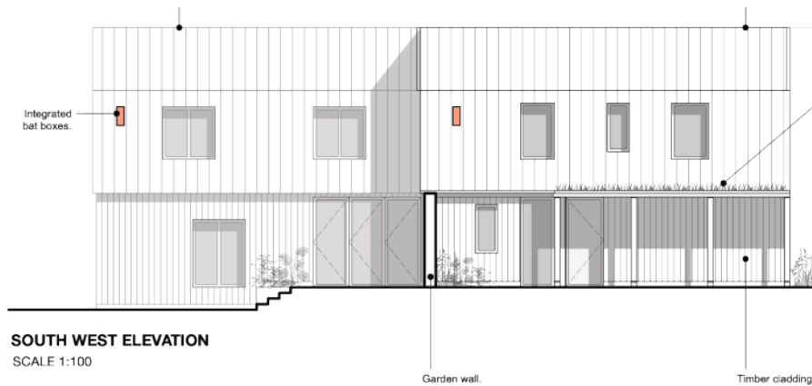
Extract from Drawing 68_P_05 - Location of integrated bat boxes (shown in orange)..
