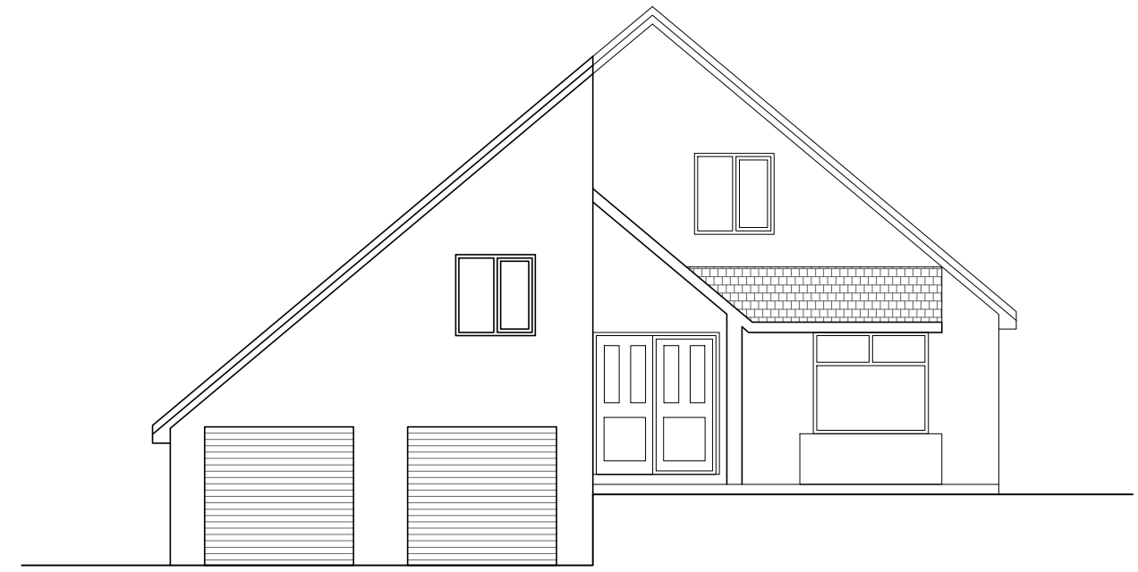
EXISTING FRONT ELEVATION SCALE 1: 100
