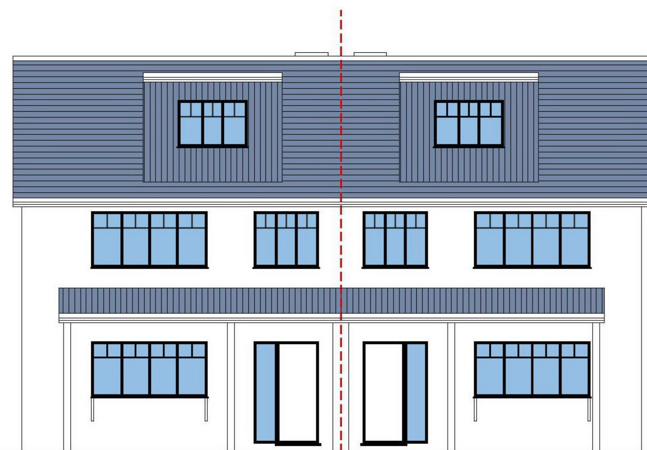
PROPOSED FRONT ELEVATION SCALE 1:100
